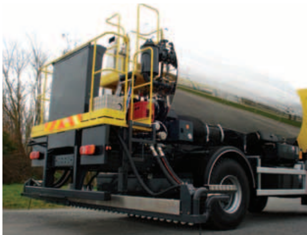
Rear control console "backup mode"
