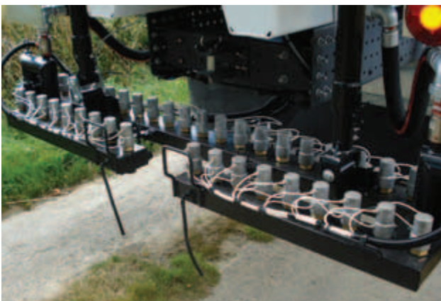
4.50m bar with toggle joints
