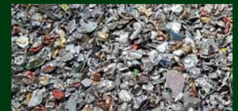
Metals from eddy current / Output metalli da eddy current
