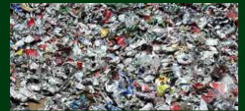
Aluminium from eddy current / Alluminio da eddy current
