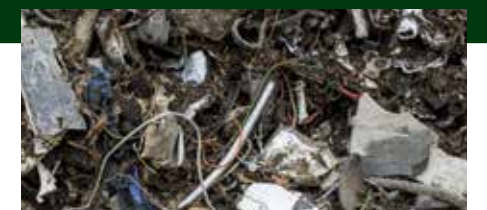
FLUFF FROM EDDY CURRENT / NON FERROSO DA EDDY CURRENT
