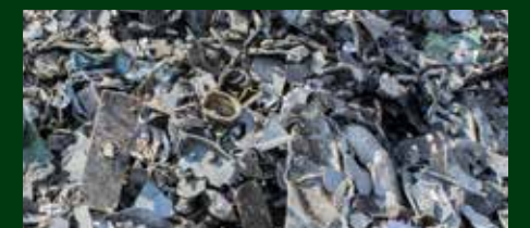
Aluminium from eddy current / Alluminio da eddy current
