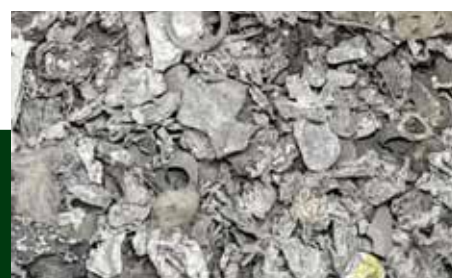
Aluminium from eddy current / Alluminio da eddy current
