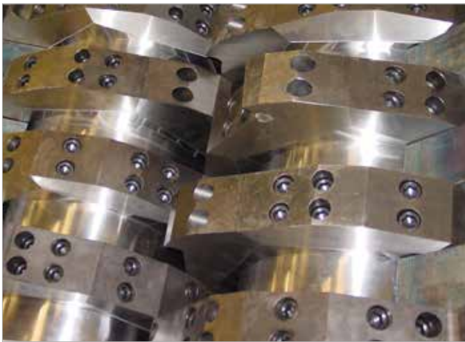
Screwed interchangeable blades / lame avvitate intercambiabili
