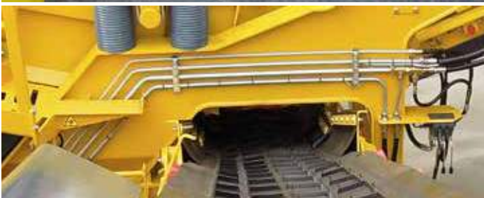
Tuberia Idraulica in metallo
